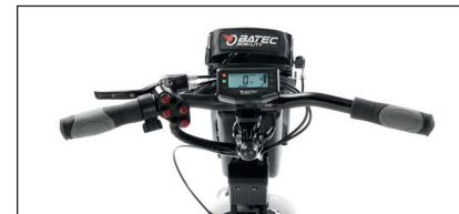
Monolever brake and accelerator handlebar for hemiplegics.
